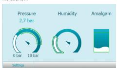
The 4,3" colour touch screen enables the monitoring directly at the Power Tower. Thanks to its network compatibility it can be monitored via the PC directly at the reception. All important parameters are constantly under control and should any failure take place they are reported immediately.
