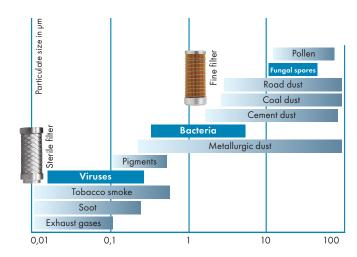
Although Dürr Dental sterile filters do not produce sterile air, they come with a 0.01  $\mu$ m filter mesh size.
