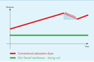
After longer operation of the compressors, moisture in the adsorption dryer increases. Yet the membrane drying unit remains dry and requires no regeneration interruption.
